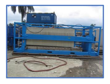
We have the DE Filter Press of 1200 sq. ft effective filtering area, which makes them very effective in handling normally required modern rigs demand. There come with either the standard 4" QC or WECO connections and are skid mounted.
