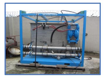
The Slurry (Mixing) Tank is dual compartment enabling simultaneous precoating and body-feeding during operations with the use of two Filter Press in parallel rig up. There also come with their body-feed vacuum pump attached. The slurry mixture is air-agitated to obtain the mixing.
