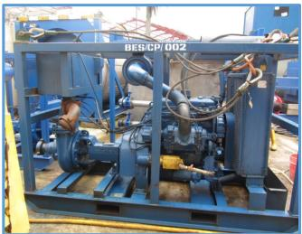
The Centrifugal Pump, with a fluid delivery rate of 15 – 18 barrels per minute, is a diesel driven pump fitted with 4" suction and discharge manifolds. All our pumps are equipped with clutches that enable engine disengagement from the pump while engine is still running. The whole unit is skid mounted
