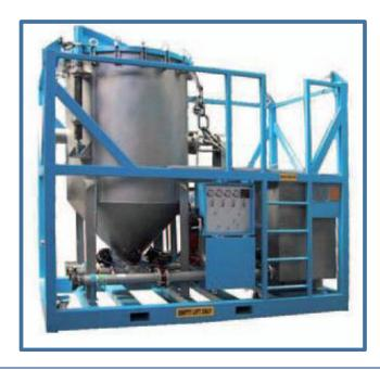
The Vertical Pressure \leaf (VPL) Units are of very high tech and quality design useful for deployment in the filtering of sea water or completion fluid when space consideration at locations is of importance. This is a 600 sq ft. effective filtration area carrying about 20 leaves. It has a maximum flow rate of 15bbl/min with a working pressure of up to 105 psi (7bar). The cleaning system is pneumatic driven with very high efficient spray nozzles.
